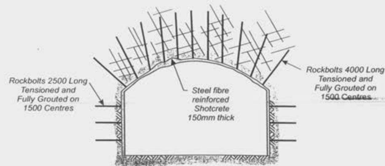
TYPICAL PRIMARY SUPPORT REQUIREMENTS FOR EXCAVATION THROUGH POOR QUALITY ROCK
