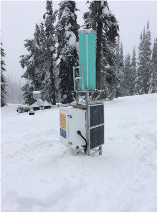
Figure 3.11 Automated snow and climate station with Campbell Scientific SR50A snow depth sensor.
