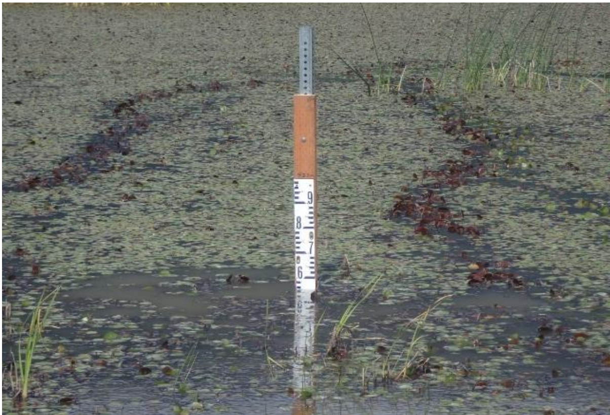
Figure 7. New staff gauge installed at WDLNA on June 1, 2016 to monitor water levels.
