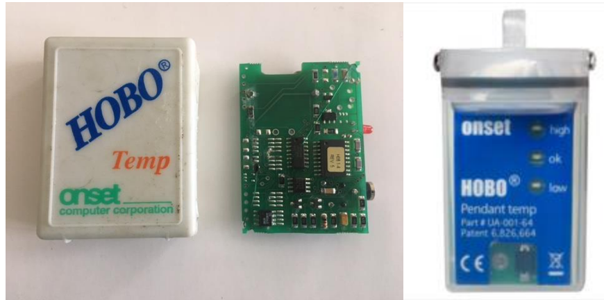
Figure 2. Temperature data logger photos (left to right): old style HOBO model H08-001-02; new HOBO Pendant model UA-001-64.
