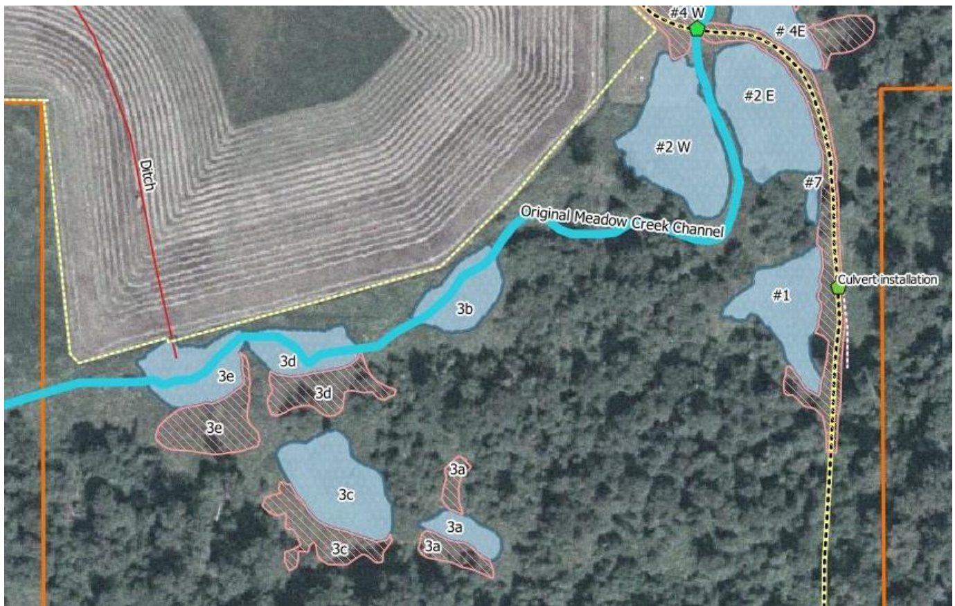
5. Satellite image showing a closeup of wetland 3e, designed to filter runoff from the pasture.
