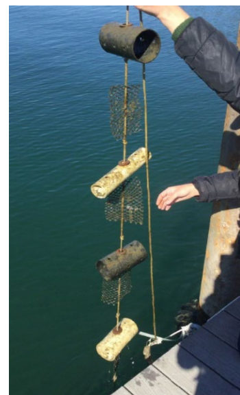
Figure 31. Substrate sampler being inspected for invasive mussel adult settlement
