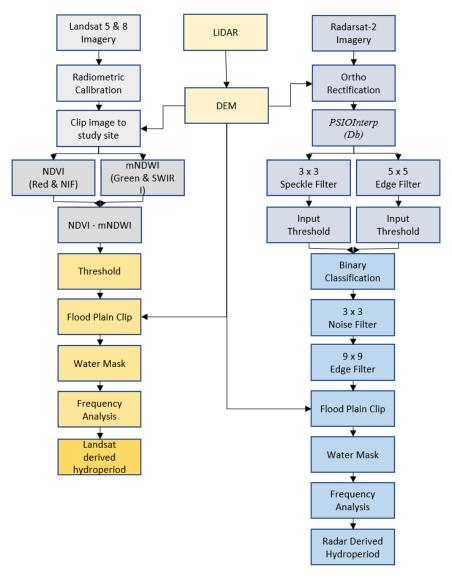
**Figure 3.** Flow diagram of (dB) thresholding and NDVI-MDWI routine to create binary water masks and hydroperiod classification. Blue rectangles indicate SAR, orange rectangles indicate optical, and beige rectangles indicate Lidar steps. SAR processing steps and filter settings follow those recommended in [51].
