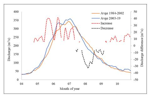
**Figure 10.** Mean daily discharge for the hydrologically active season (April to October) for T1 and T2. Increases or decreases in flow from T1 to T2 are illustrated for differences >5 m<sup>3</sup>s<sup>-1</sup>.
