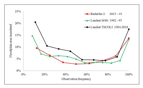
**Figure 9.** Comparative hydroperiod (open water area frequency) for Landsat TM/OLI (n = 61), SAR (n = 8) and MSS (n = 12). (Note, the 0% hydroperiod frequency is not illustrated due to high variability across the three methods; see Tables 2 and 3).
